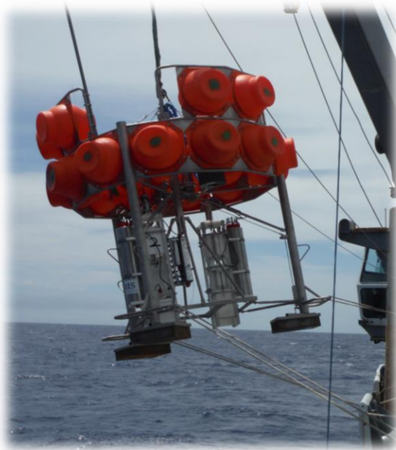
2. The 'Yu-Yu' camera system used in this study showing the camera housing, strobe, bottom contact switch and trigger weight.
